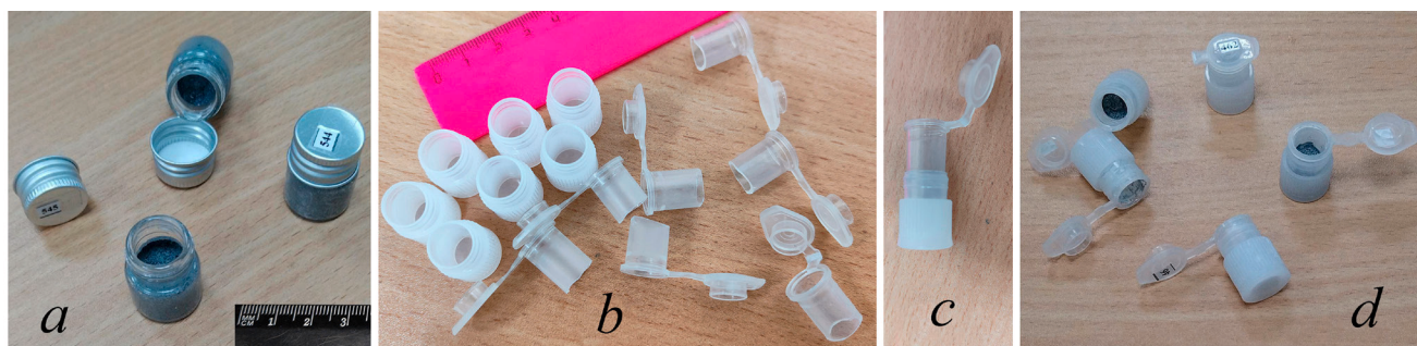
Fig. 1. Vessels used for laboratory culturing of oribatid mites: a – glass jars with screw-on lids for group culturing of adults, b – plastic specific lids and cut Eppendorf tubes, c – partially combining specific lids and cut Eppendorf tube, d – completed plastic chambers for individual culturing of juvenile instars
