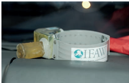
Figure 50. “Pulsar” radio transmitter (manufactured by ZAO “S-PAS”) (Photo by A.L. Salman).
